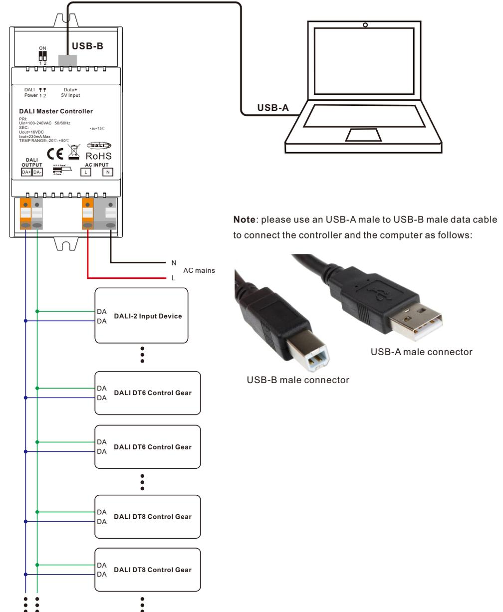
**Note:** When use built-in DALI power supply, please dial both DALI power setting dip switches to "ON" position. The controller can supports up to total 64 control gears and 64 DALI-2 input devices.
